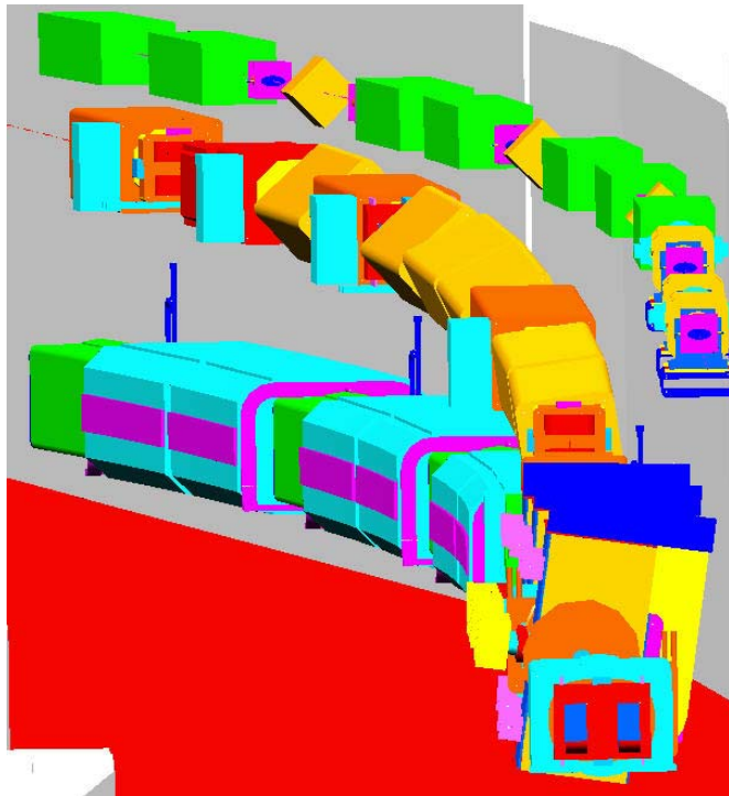
Drawing of the NuMI extraction line coming out of the MI below the Recycler
