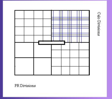
To keep the timing gates for each Photon Barrel Veto (PBV) section as narrow as possible, it is necessary to use the natural divisions of both the PR and Calo for the L0 trigger
