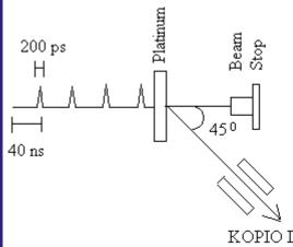
BNL AGS supplied proton beam on a Platinum target
