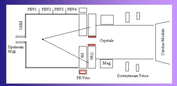
Reconstructed  $\pi^0$  vertex must be 50cm downstream of the decay tank entrance and 50cm upstream of the PR, due to expected neutron background
