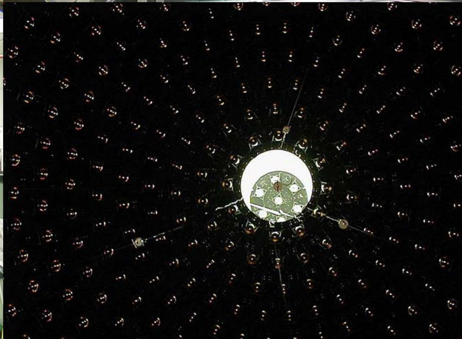
Pattern of hit tubes (with **charge** and **time** information) allows reconstruction of track location and direction and separation of different event types.
