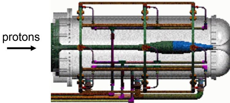
170 kA in 140  $\mu$ sec pulses @ 5 Hz
