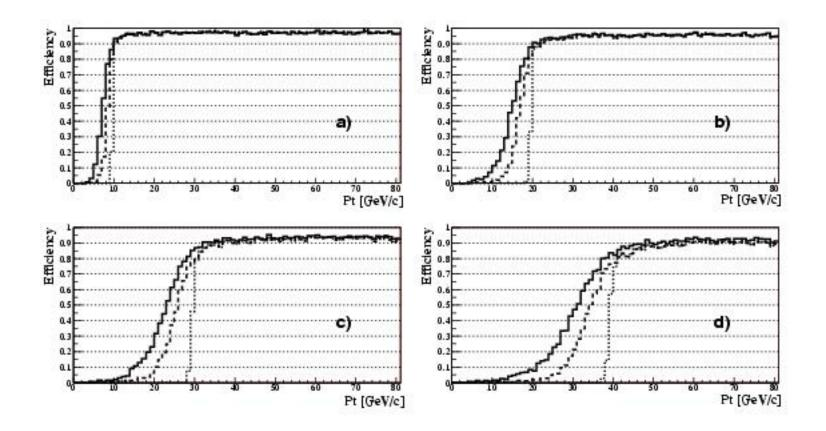
Cumulative efficiency for single muons to pass the Level-1 (solid), Level-2 (dashed), and Level-3 (dotted) triggers as a function of the generated  $p_T$  for several trigger thresholds: a)  $p_T>10~{\rm GeV}/c$ , b)  $>20~{\rm GeV}/c$ , c)  $>30~{\rm GeV}/c$ , and d)  $>40~{\rm GeV}/c$ .
