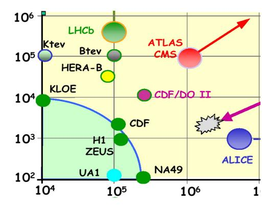
• Event size (bytes) versus Level-1 Trigger Rate (Hz). • ATLAS/CMS High number of channels/bandwidth (500 Gbit/s). • LHCB High Level-1 trigger. • ALICE Highest event size/data archive.
