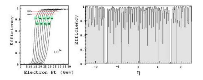
The efficiency of the Level-1 trigger for single electrons as a function of the electron  $p_T$ . On the right, the efficiency, as function of  $\eta$ , for electrons with  $p_T$ =35 GeV/c.
