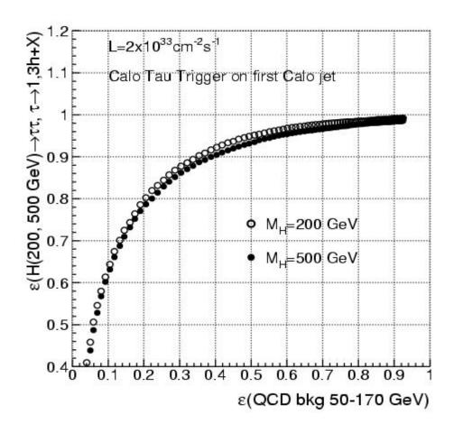
Efficiency of the  $\it Calorimeter~Tau$  trigger when applied to the first calorimeter jet in  $\it A^0/H^0 \to \tau\tau \to 2\tau$ -jet and QCD di-jet events.  $\it M_H=200$  and 500 GeV/ $\it c^2$  for  $\it L=2\times 10^{33}\, {\rm cm}^{-2} {\rm s}^{-1}$ .  $\it P_{isol}=\sum \Delta R < 0.4\, E_T - \sum \Delta R < 0.13\, E_T$  is varied between 1 GeV and 20 GeV in 0.2 GeV steps.
