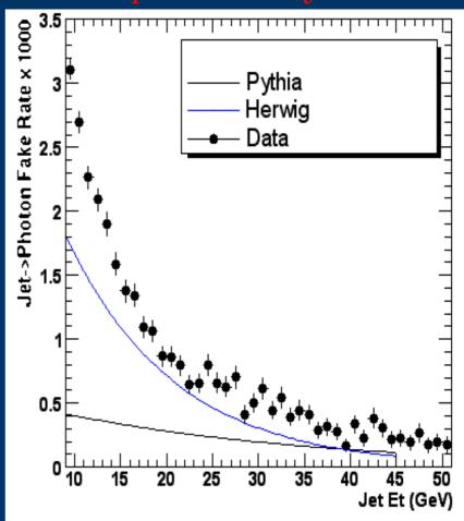
At TeV Jet  $\rightarrow \gamma$  miss ID is obtained from  $\gamma$ +jet data. We should evaluate how does it work with LHC detectors
