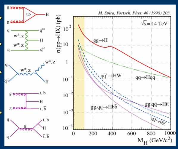
Having available four production mechanisms is a key for measurements of Higgs parameters
