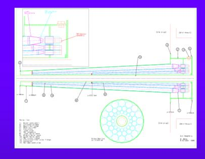
36x [4.8mm Pb + 6.4mm Sc] Liquid scint + wls fibers 18 Ham R5900 PMT each end
