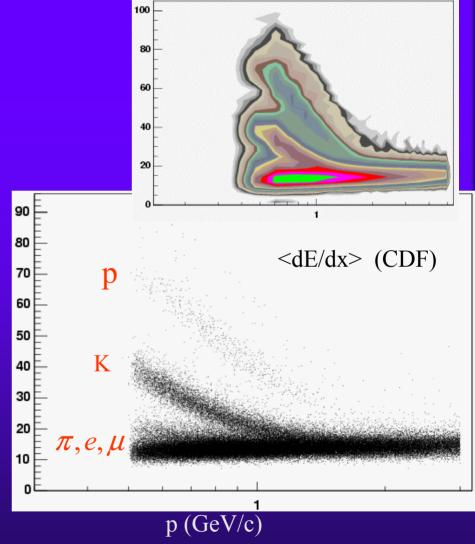
Low p\_T particles in range  $\sim 0.3 - 3.0$  GeV/c, high identification probability
