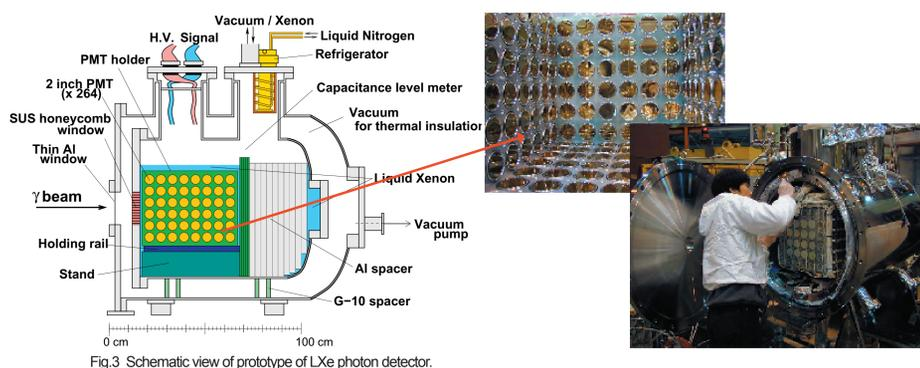
Fig.3 Schematic view of prototype of LXe photon detector.
