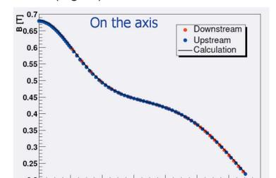
Fig.11 Measured magnetic field along magnet axis. Calculated magnetic field is also shown with a solid line.
