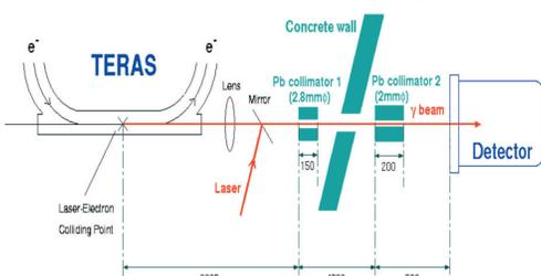
Fig.4 Layout of the beam tests at the laser Compton backscattering facility at TERAS electron storage ring in the AIST, Tsukuba, Japan
