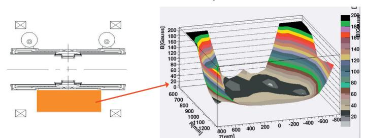
Fig.12 Measured stray field around the photon detector region.
