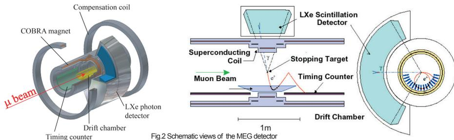
Fig.2 Schematic views of the MEG detector
