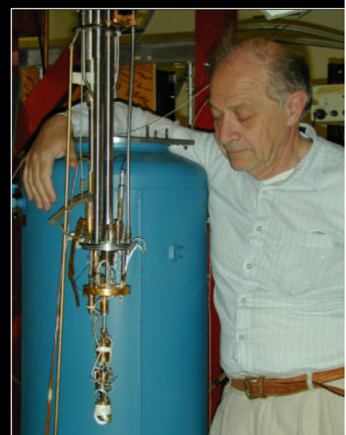
Oscar Vilches and his dilution refrigerator.
