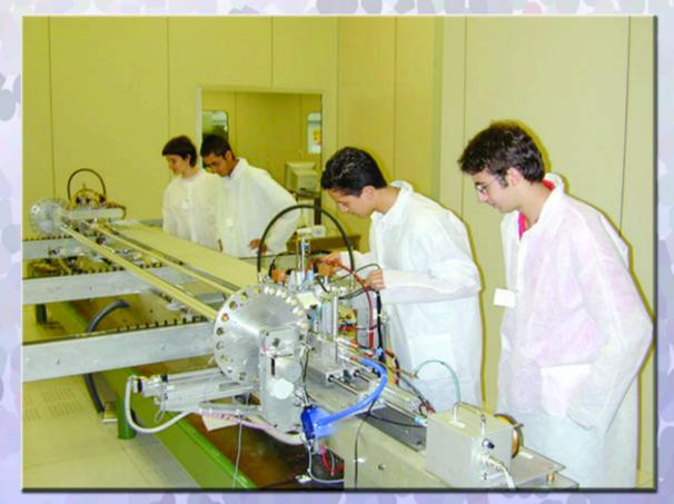
Physicists, engineers, and technicians unite physics and technology in the development of advanced detectors for next-generation experiments. The photo above shows the assembly of Monitor Drift Tubes, which are large detectors for charged particles that will cover an area of about 5000 m<sup>2</sup> in the TLAS experiment at CERN.
