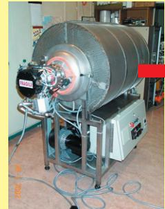
Vacuum oven for out-gassing of power couplers
