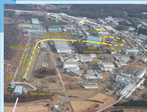
Bird's-eye view of the neutrino beam-line at KEK. It provides a 98% pure wide-band < E_\mu > 1.3 \text{ GeV} muon neutrino beam from the KEK 12 GeV PS. A near detector system is located 300 m downstream from the target.
