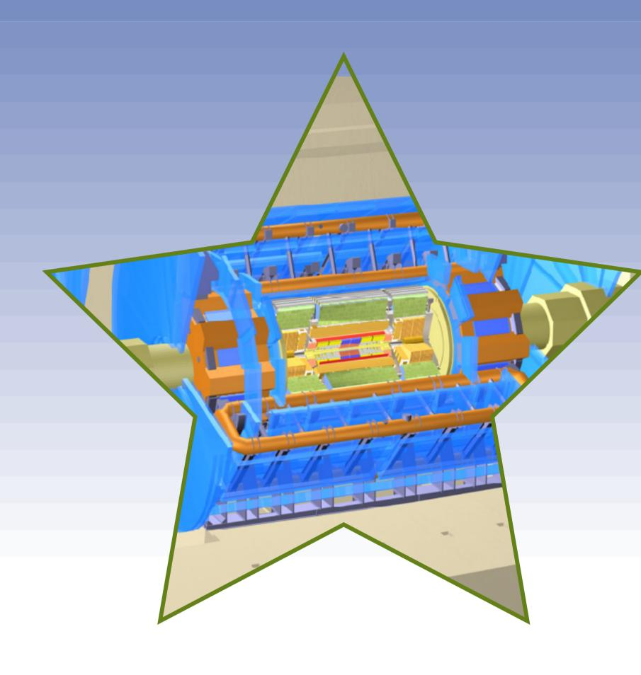
While CERN builds the accelerators, scientists from universities and research institutes build the detectors. As physics has advanced, detectors have become bigger and more complex. The largest of those in preparation for the LHC stand as high as a sixfloor office block. They weigh up to 12500 tonnes, and are being built by teams of almost 2000 people. Altogether, CERN's research programme involves some 6500 researchers from 500 institutes in 80 countries.
