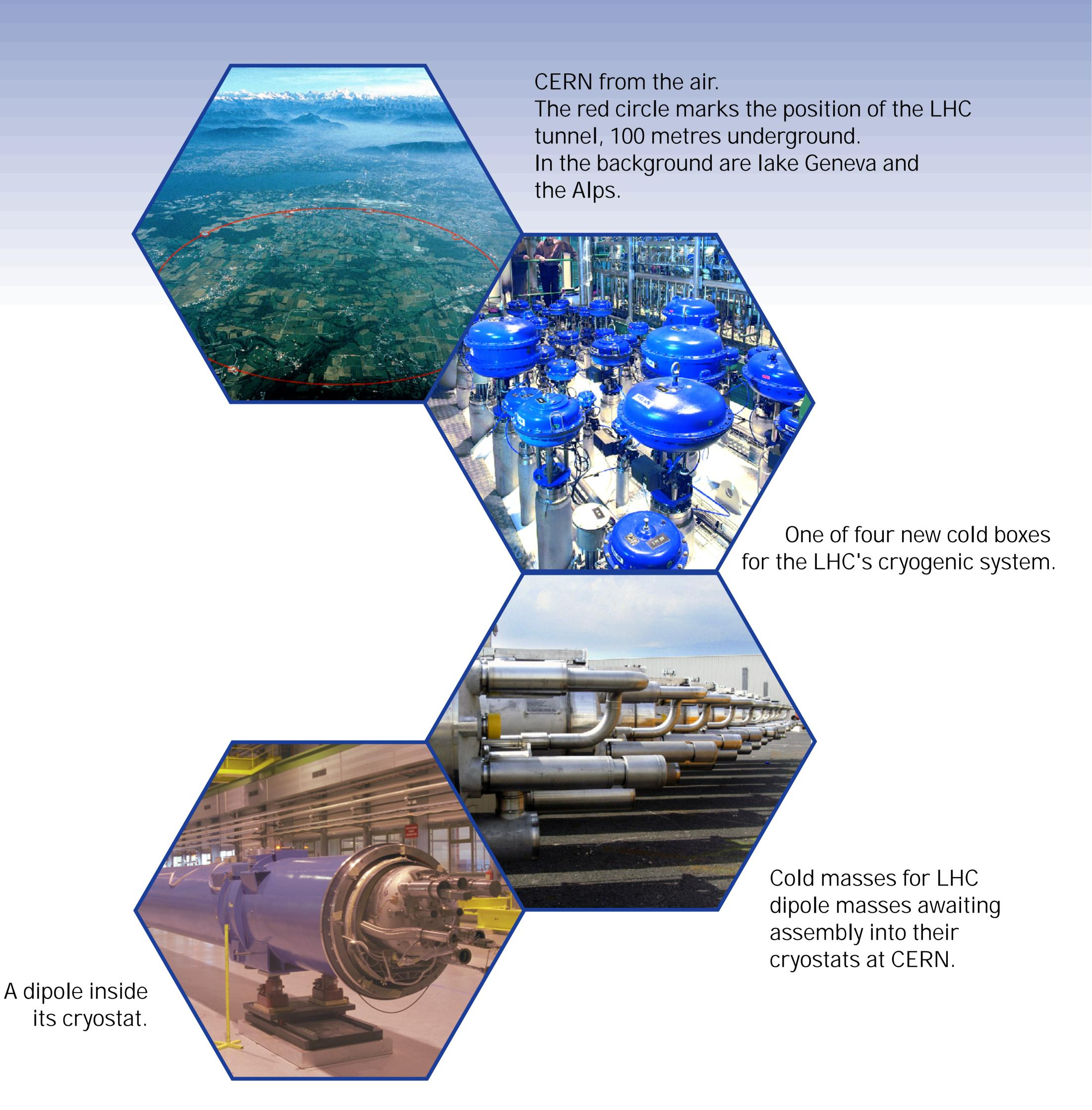
The LHC superconducting magnets will generate the highest magnetic fields ever reached in an accelerator of this scale. The dipoles and quadrupoles will be interconnected so as to form a continuous cryogenic "pipe" installed in the 27 km-long LHC tunnel with a separate cryogenic distribution line. The superconducting RF accelerating cavities, along with the beam cleaning and beam dump systems, will complete the machine.
