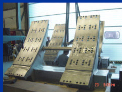
Modules in the region of the saddles simply rest on swivel bolts which are mounted in the holes shown.
