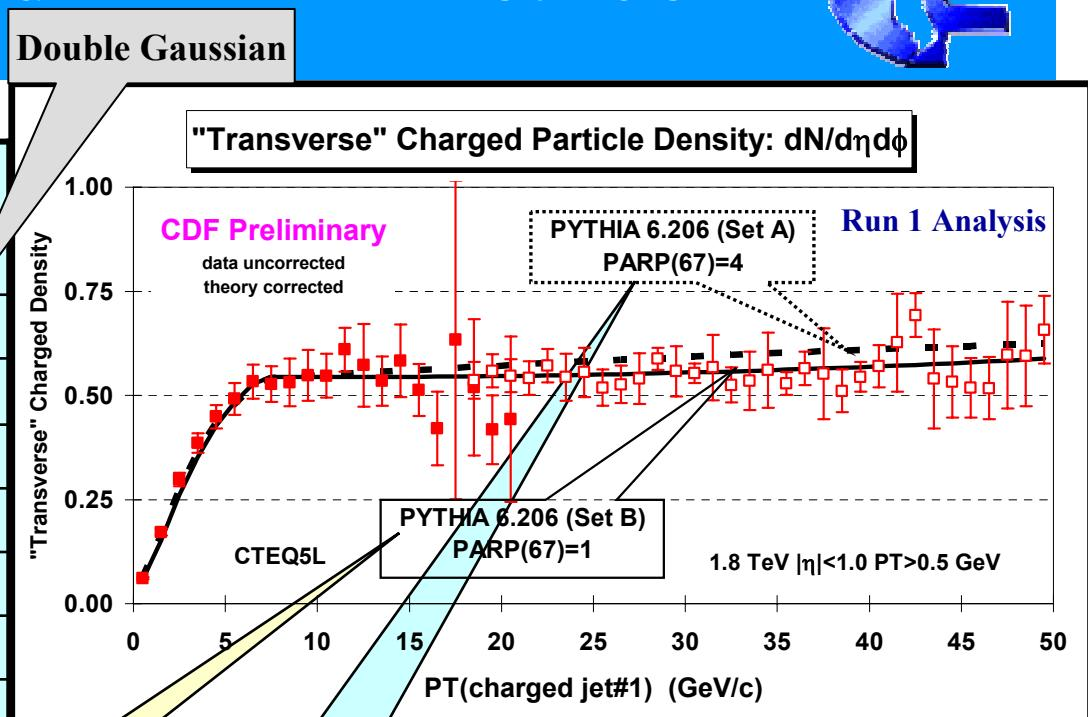
Plot shows the "Transverse" charged particle density versus  $P_T(\text{chgjet}\#1)$  compared to the QCD hard scattering predictions of two tuned versions of PYTHIA 6.206 (CTEQ5L, Set B (PARP(67)=1) and Set A (PARP(67)=4)).
