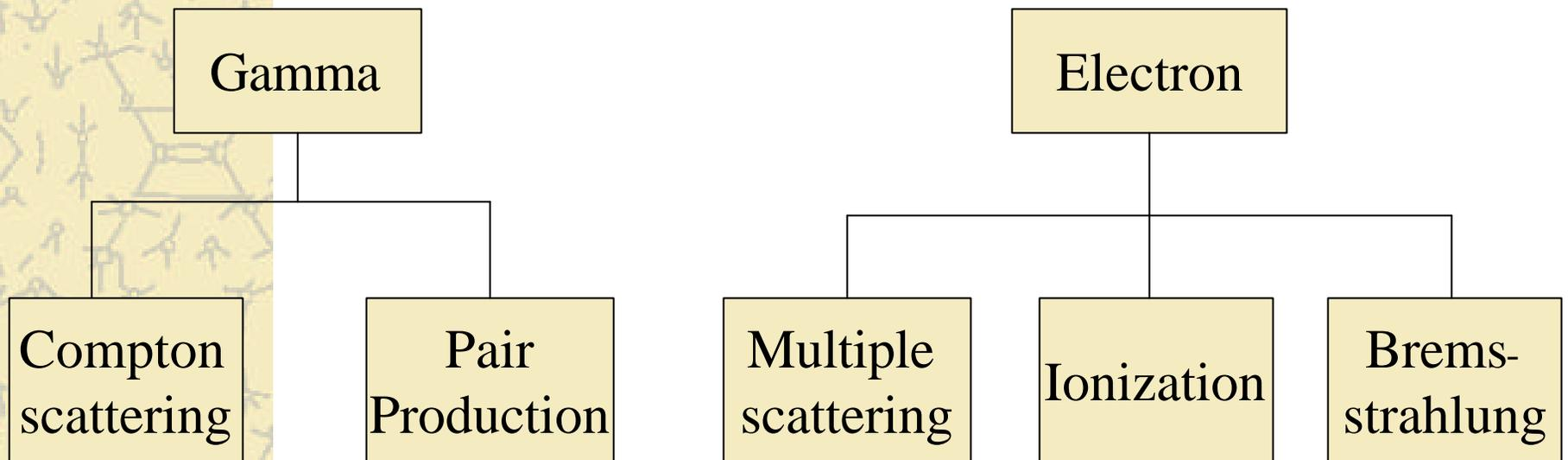
Each particle class has a process manager to which physics processes are registered
