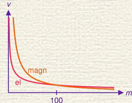
Voltages are independent of mass (for an ion source on a given potential), which makes injection of rare ion species simple
