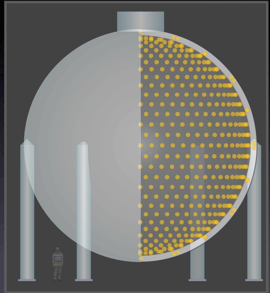
Detect neutrino interactions via  $\check{C}$  and scintillation light
