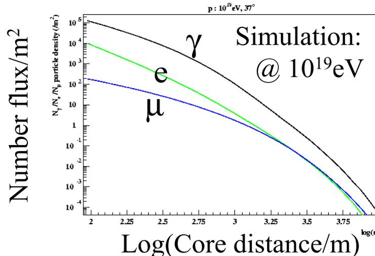
Sample the particle flux using sparse arrays of scintillators or water Cherenkov tanks. **Signal  $\sim E$ .**
