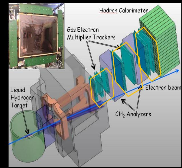
GEM for the Super BigBite Spectrometer for 12 GeV Experiment @ JLab
