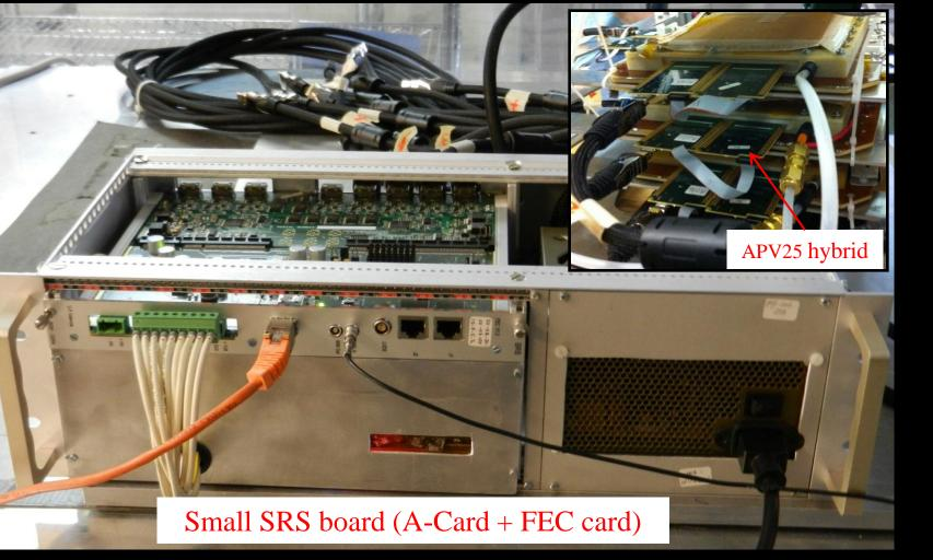
APV25 based SRS small system @ University of Virginia the system has up to 2048 channels to read out 4 tripleGEM detectors  $(10 \times 10 \text{ cm}^2)$
