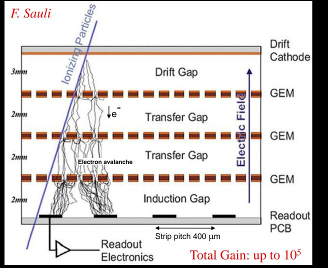
A triple-GEM detector: gain sharing between the foils improves the reliability of operation at high gain
