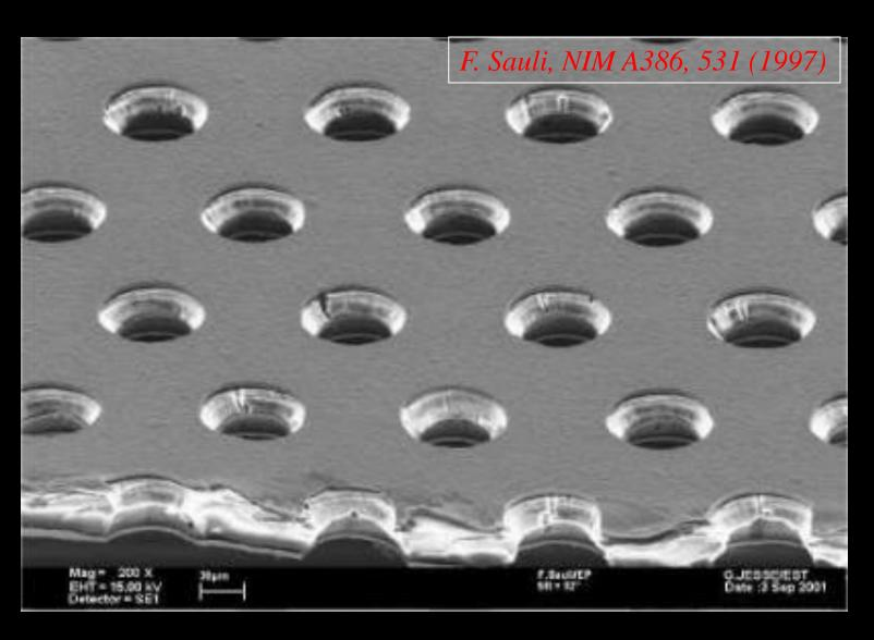
GEM foil under electron microscope
