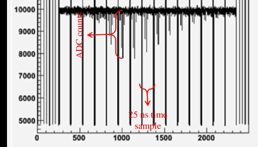
APV25 raw data: 25 ns time samples of the ADC analog signal
