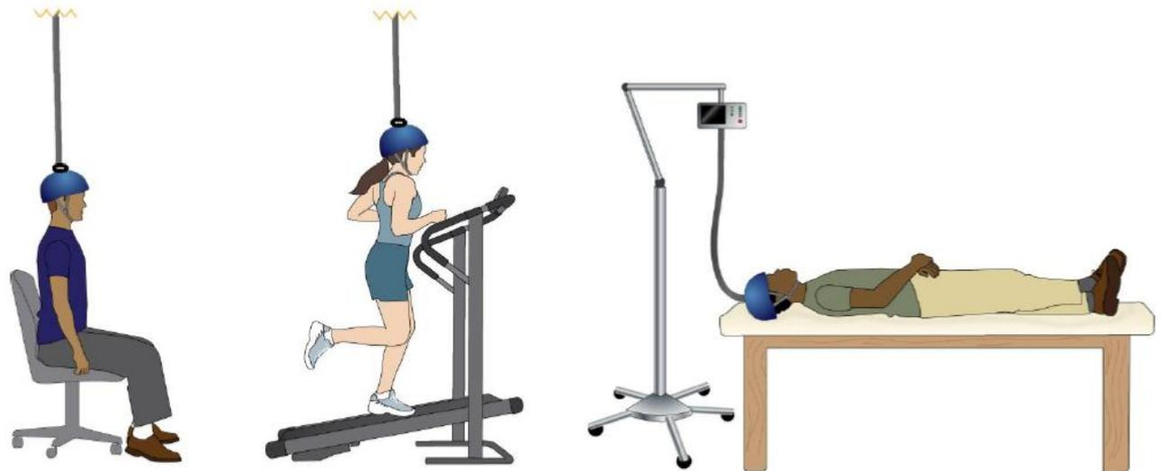
Examples of some possible situations with patients wearing the imager helmet: sitting in a chair (*left*), exercising (*center*), and laying down on a bed (*right*). Another option with a (helium) balloon supporting the weight of the helmet, allowing for even more movement freedom during imaging session, is not shown here. Except for the case of a patient on a bed, the helmet is suspended by a flexible harness /suspension attached to a hook on the helmet.
