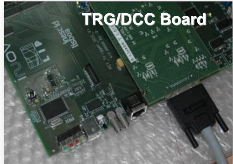
L1 Trigger/DAQ system is housed in a single crate with two dedicated buses
